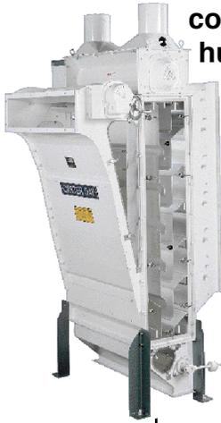
The Duo-Aspirator is a medium capacity aspirator that separates light material from heavy material. A vertically rising air stream lifts light material out of the air
