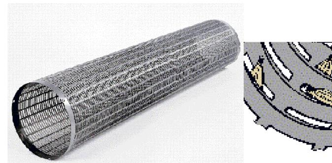
**TRI-BAR** - The Carter Day Tri-Bar slotted cylinder can double the cylinder capacity depending on slot width. The Tri-Bar operates by using a triangular shaped wire, instead of punched slots, producing more open area. Rigid construction maintains opening tolerance longer. Slot widths are available in sizes from 2.5/64 inch (1mm) wide to 36/64 inch (14.3mm) wide. Best for separating particles by thickness with high capacity.
