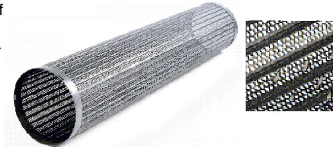
**FUNLSIZER®** This patented cylinder is the latest in technological design. The perforations are funnel shaped round holes. The funnel design upends the grain directly into the hole and either allows passage through the hole or rejects the grain and passes it down the cylinder. The funnel style holes are available from 13/64 inch (5.2mm) to 23/64 inch (9.1mm) in diameter. Best for separating large particles by width.
