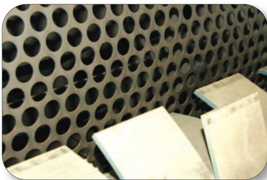
The Rotating Scalping Reel is constructed of a stainless steel perforated screen. The round hole perforated screen design eliminates blinding of the scalping reel.
