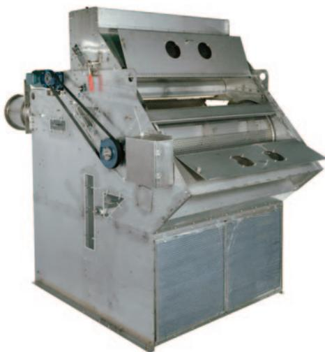
The Stainless Steel Scalperator features scalping and aspiration in a single machine providing a high capacity and efficient method for removing streamers, agglomerates and fines in a single pass, surpassing the capabilities of traditional elutriators.
